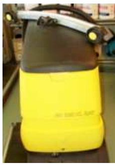
BR 530XL 21" CYLINDRICAL BRUSH FLOOR SCRUBBER
